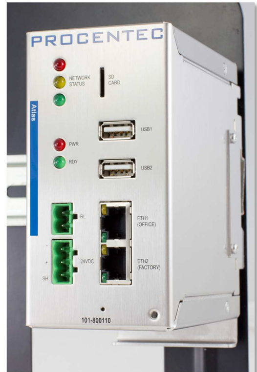
Figure 1 – Atlas mounted on a 35mm DIN
